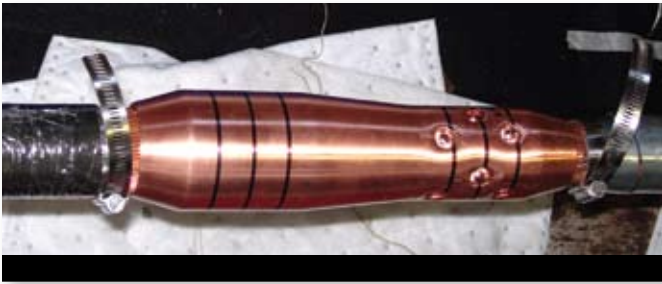
A connector is used to accommodate the transition between two different cable conductor sizes.
